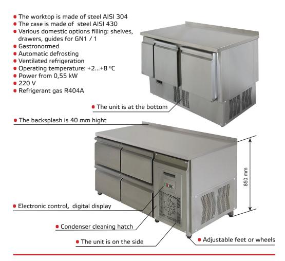
All refrigerating tables **SIMECO** can be made with swing doors and drawers. There are various options for internal filling and custom sizes of products.
